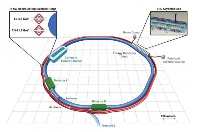
A schematic of the world's first electron-ion collider (EIC). Adding an electron ring (red) to the Relativistic Heavy Ion Collider (RHIC) at Brookhaven would create the eRHIC. Image credit: Brookhaven National Laboratory-CAD eRHIC group.
